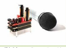
3D AudioSense acoustic sensor system prototype
